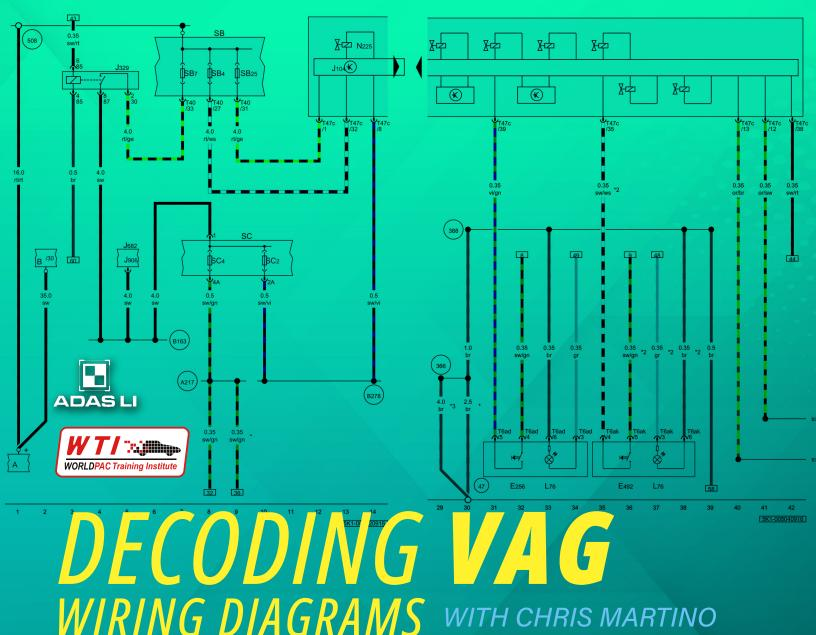
VW and Audi diagrams are different, not impossible. Understanding VAG track-style diagram organization and DIN conventions, component IDs and current-flow tracks. How to read tracks left to right and top to bottom to plan tests, find splice points and confirm root cause.
